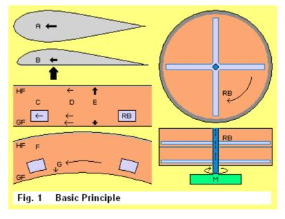
The motion process is comparable with a tracked vehicle. A chain link is laid down at the ground in front of the vehicle and keeps that position. When the vehicle did roll over, the link is accelerated upward and is flying forward, by double speed, all over the vehicle. Opposite here, the stick-face functions like rough asphalt and the air is flying along the glide-face with accelerated speed (see arrows at D).
