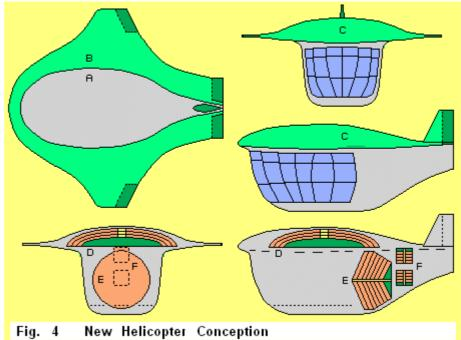
reduced to the rear end. The contours (B, green) of the helicopter reaches out over the cabin at the front side above the bow, aside flat merging into short wings, also flattened out to a wide fin at the rear end. So the top of the helicopter builds a wide and rounded dome C.
