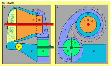
Pump is installed quite downside of tank, so water is transported e.g. for starting system. At running mode, strong suction exists from the turbine and the turbine-inlet backward, so pump won't demand much energy-input for drive but will turn just idle within that flow. At the other hand, any acceleration of pump revolutions, immediately will increase mass-throughput and thus also performance of turbine.
