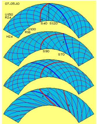
surface meet two flows: at the one hand forced movement within canals and at the other hand free flow of water alongside cone-wall. At third jacket of that picture again these canals L (red) are drawn several times and now also tracks D (blue) of free flowing water. Both cross about right-angles.
