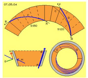
Diagonal movement M schematic is drawn once more left side. Inertia all times shows straight ahead in movement direction, here thus diagonal-ahead towards inner wall. Redirection of flow results centripetal acceleration resp. centrifugal forces onto inner wall. That wall can take force G only right angles to its surface, so force-component H results, parallel to wall, much stronger than at upside example of rotation at steady height.
