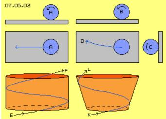
At this picture right side once more bowling ball B is sketched, again rolling at plane towards left. Now however that ball got overlaid additional turning movement C, cross to its forward movement. Bended track D results (like any bowling-fan perfectly demonstrates).
