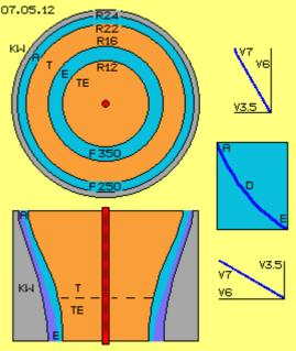
horizontal direction only by 3.5 m, however exits outlet by vertical speed of 6 m/s (see the vector-graphs).
