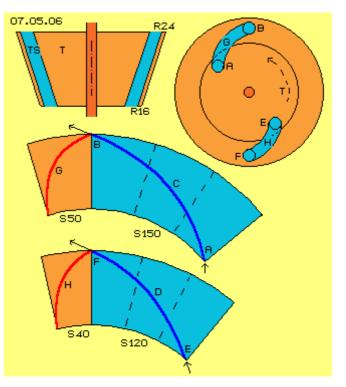
canals naturally press also at outer walls, due to centrifugal forces. Starting at certain speed, thus also these water masses become lifted upward. If canals allow that additional motion upward-outward, water upside will flow off outlet by angle more acute.
