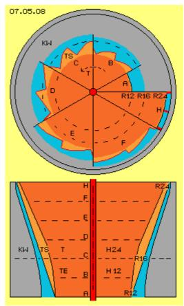
At longitudinal cross-sectional view are marked diverse axial levels by dotted lines A to H. Upside at picture 07.05.08 these cross-sections are partly drawn, each by a sector, one level aside next level. At downside end A of turbine-inlet, radius is 12 cm and ring-shaped cross-sectional surface is available for water between round turbine and round cone-wall (here drawn within a sector of 30 degrees).
