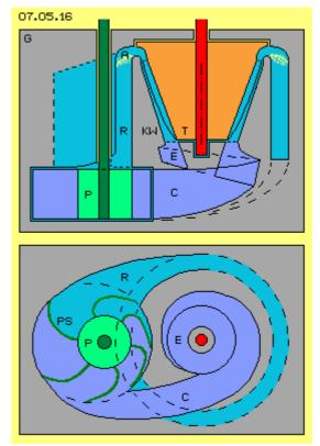
It's also possible, total inner space of machine could be filled up with water, also at area of outlet A, so closed circuit of water exists. That machine naturally could again be arranged with horizontal shaft. Above this, that general principle of movements could be realized by most different variations.
