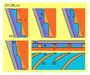
thus move faster in turning sense of system, i.e. sweep over canals. Within canals thus comes up spinning movement C, increasing pressure onto pressure-sides of canals. So also these free-flowing parts of water indirectly contribute to turning momentum.
