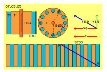
Water downside turns e.g. by 6 m/s just as fast as turbine (see arrows V 6 and T). Water e.g. enters by angle of 30 degrees upward into canals. Vertical speed thus is about 3.5 m/s (green arrow V 3.5), diagonal speed thus is about 6.9 m/s (blue arrow V 6.9).
