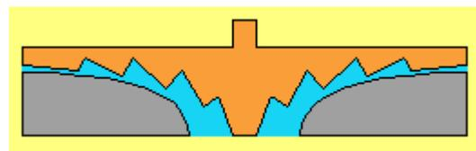
One can clearly see, the teeth growing off at the centre and there at first makes the fluid turning. Afterward, the suction sides become wider and tilt towards outside.
