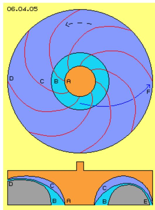
Downside at the longitudinal cross-sectional view at left side, the outlet D is arranged aside of the machine. As an alternative at right side is sketched, the canal well could be arranged within a half circle, so the blades C practically are embedded within a 'bowl' and the outlet E shows back into axial direction. This arrangement could be especially advantageous, if the dent-shaped blades are used at a turbine.
