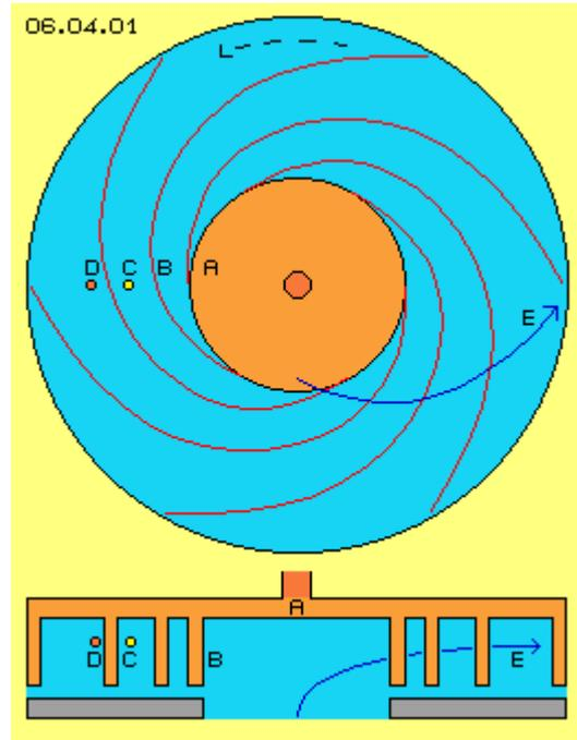
An other particle C (yellow) is drawn near the rear face of the blade. The fluid there is pressed ahead-outward indirectly by the following wall and the neighbouring fluid. At the other hand, that wall moving forward affects suction and the particles fall into these 'empty' areas without resistance. So the generated flow only partly is produced by mechanic pressure, because particles partly fall into the wanted direction by their 'own movement energy'.
