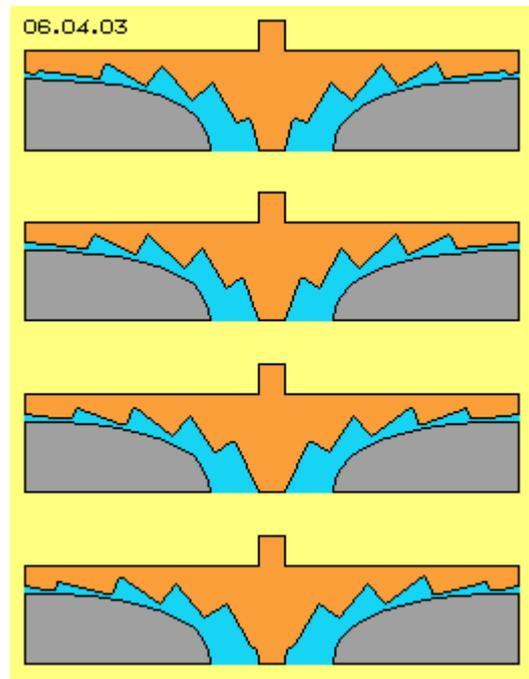
The suction sides of that rotor still are spiral bands (analogue previous picture 06.04.01), arranged some tilted. These bands can be long-winded or can run more radial direct from inside towards outside. The cross-section all times shows these teeth-like steps, however the flow is running diagonal and thus the teeth appear more stretched into flow direction.
