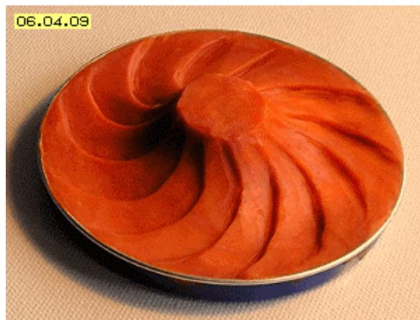
Picture 06.04.09 shows a model of a turbine-rotor (without corresponding faces of a housing). The blades are shaped like 'horseshoes', embedded within the round deepening of the rotor. The inlet flow enters the rotor all around form outside diagonal inward. The outlet flow is running off near the center in axial direction.
